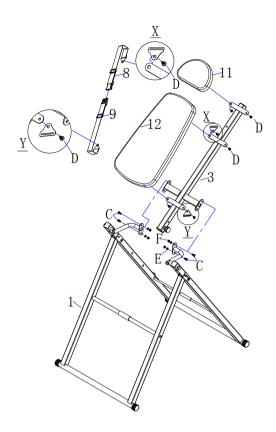
A.Use screws (D) to attach the Headrest pad11) and the Back pad (12) and at the same time install the webbing (8) and webbing (9) in the X and Y pictures on the iron sheet on the Backplane (3).
