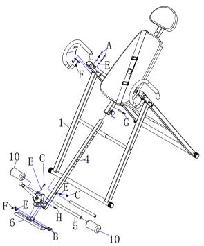
A. Insert the foam tube (5) into the large hole on the height adjustment frame (4), and fix it with screws (C) and flat washers (E). Put the foam (10) into the foam tube from both ends (5) on;
